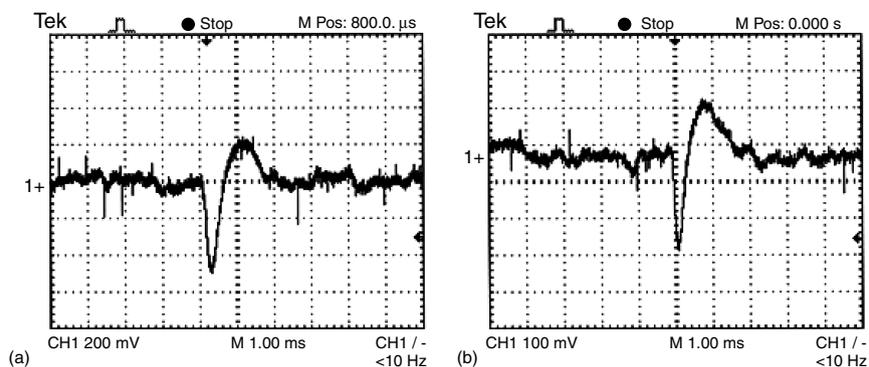
**FIGURE 12.4** Comparison of electrodes for measuring electrophysiology. (a) Saline-filled glass micropipette; (b) CFM. Both recordings were collected in the dorsomedial caudate–putamen of a urethane-anesthetized rat.
