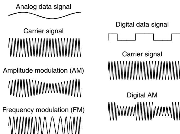
**FIGURE 12.6** Modulation. (Modified from Weisman, C. J., *The Essential Guide to RF and Wireless*, Prentice Hall, Upper Saddle River, NJ, 2002.)
