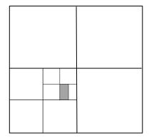
In the map or diagram above we start with the last item (the south-west quarter) listed in the description, which is the largest measure given, and work backwards to the smaller/more specific measures.
