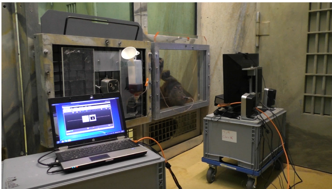
Figure 2. Eye-tracking setup. An infrared eye-tracker non-invasively records an orangutan's gaze as she attends to pictures and videos presented on a monitor, just outside of her enclosure. A nearby laptop controls stimuli presentation. Subjects voluntarily approach the setup to view the stimuli and sip a slow stream of juice. Copyright: Christopher Krupenye and Leipzig Zoo.
